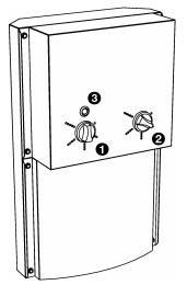
The operation of the control unit depends on the function option chosen, the control components connected, and on the positions of the switches **①** and **②**.
