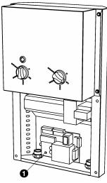
**3** Press the reset knob **0** on the PCB.
